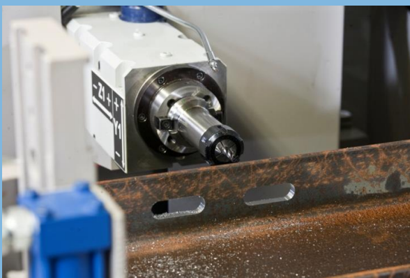
Oblong holes milling
